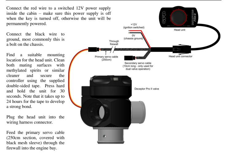
Often there is an existing grommet that can be used for this purpose. In any case, it is important to ensure that the lead is protected where it passes through the firewall to prevent wear or damage.
